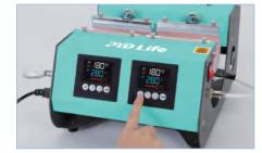
Set the parameters for each of the two control panels according to the needs of the mugs;
