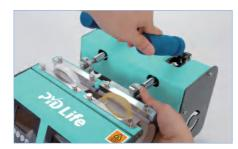
Adjust the pressure with the pressure knobs separately, press the mugs to find the proper pressure;
