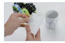
Fix the printed images on the mugs individually with the heat resistant tape;
