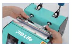
2 Adjust the pressure with the pressure knobs, press the tumbler to find the proper pressure;
