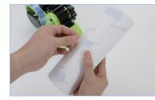
1 Fix the image on the tumbler tightly with thermal tape;
