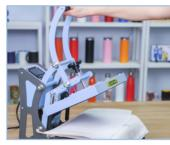
After countdown, lift up the handle to open the heat platen;
