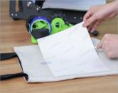
3 Fix the image on the printed item with thermal tape;
