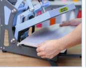
2 Put a piece of protective paper on the silicon mat, so the inks won't ruin the silicon mat and the printed items;
