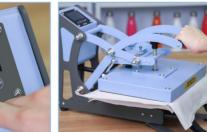
7 Set printing time and temperature, and wait for the machine to heat up;
