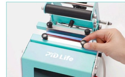
5 Fix the new heater with the screws in the amount it needs;
