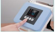
Set printing time and temperature, and wait for the machine to heat up;
