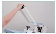
8 After the countdown, the machine will beep a sound and then lift up the handle;
