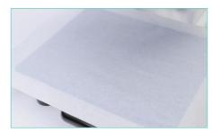
Put a piece of protective paper on the silicon pad so that the inks won't ruin the silicon pad and the printed items;
