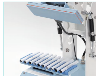
2 Put the pen on the machine, lined up neatly with the print side facing up;
